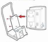
Using the thumbscrews, secure the rear panel of the BP device to the stand.
